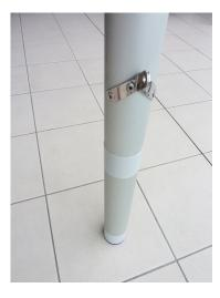
Reason for change: To clarify that mast step abrasion tubes or collars may be in separate pieces.
